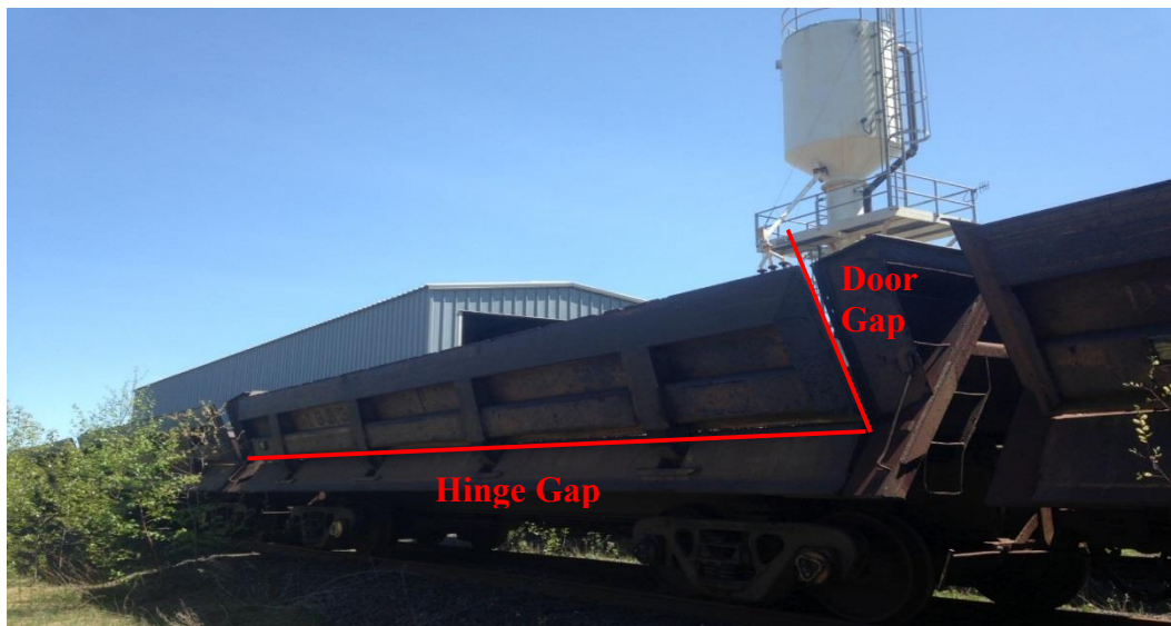
Figure 2. Photo of Side-Dumping Rail Car with Gaps Highlighted
